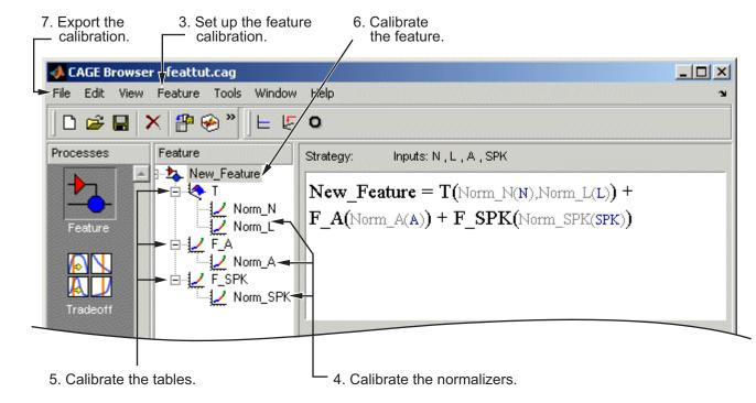
The normalizers, tables, and features form a hierarchy of nodes, each with its own view and toolbar. The feature view is shown.
