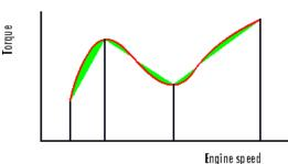
Optimizing the position of the breakpoints can greatly reduce the error between the interpolated table values and the model.
