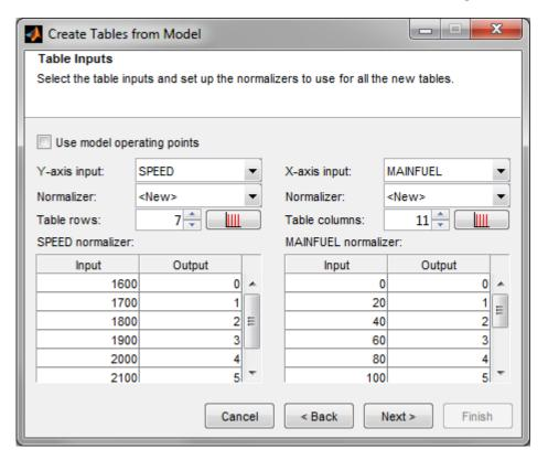
You must specify the breakpoints for your model input normalizer. Edit breakpoints by clicking the button after **Table columns**, and enter a number of points and the range to space the breakpoints over. If you do not do this, model inputs are spaced over 0-1, because CAGE cannot determine the range automatically as happens with variables. After you create your tables with a model input, in the Variable Dictionary
