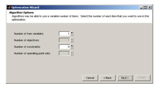
The fmincon algorithm can only have a single objective, so this control is not enabled. Choose the number of free variables and constraints you require. You can also add constraints later.
