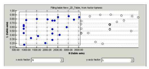
3 To fill the table based on an extrapolation over these data points only, click Fill Table.
