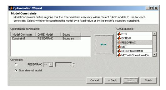
Select a model for each constraint by selecting a CAGE model and a model constraint and clicking the button to match them up.
