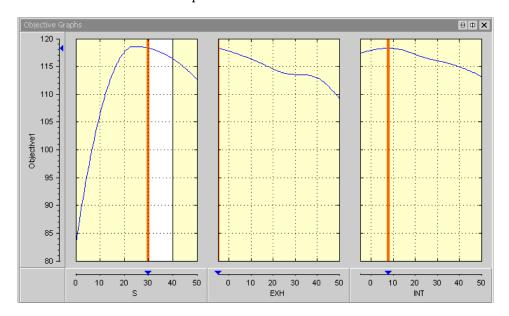
The Objective Graphs show cross-section plots of the objective function against each free variable in the problem. The left plot is a plot of the objective function against S, with EXH and INT at their optimal values, for the second run. The range constraint for the second operating point ( $30 \le S \le 40$ ) can be seen; within the constraint region is white, and all other regions outside the constraint are yellow.
