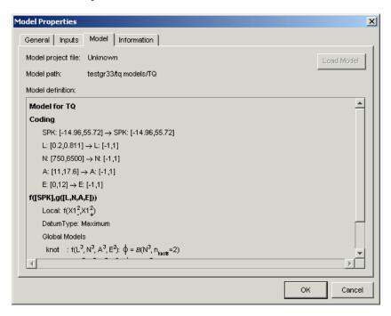
Here you can view the model definition, the project file, and the model path. Function model definitions are shown here. For MBC models the model definition (showing the parameters and coefficients of the model formula) is the same information you would see in the Model Browser part of the toolbox when selecting **View > Model Definition**.
