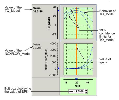
Performing a tradeoff calibration necessarily involves the comparison of two or more models. For example, in this case, the tradeoff allows a calibrator to check that a value of spark that gives peak torque also gives an acceptable value for the NOX flow model.
