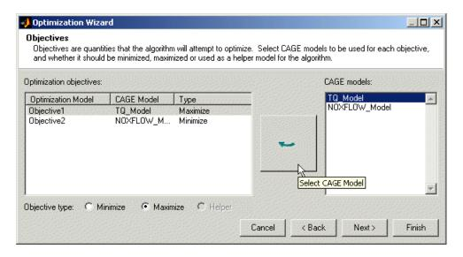
Here you can select which models from your session you want to use for the optimization, and whether you want to maximize or minimize the model output. The fmincon algorithm is for single objectives, so you can only maximize or minimize one model. The NBI or gamultiobj algorithms can evaluate multiple objectives. For example, you might want to maximize torque while minimizing NOX emissions. Remember you can also define constraints later, for example, using emissions requirements.
