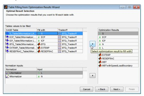
Verify the **Normalizer inputs** show the correct inputs. You might need to specify the **Normalizer inputs** to match with optimization results, if you are filling tables with different inputs to your optimization operating points. See "Table Filling When Optimization Operating Point Inputs Differ from Table Inputs" on page 7-13.
