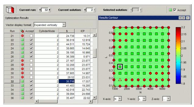
2 To see which mode is selected as best for all operating points in one view, switch to the Selected Solution view. Select View > Selected Solution or use the toolbar button. The table and contour plot display the selected best solution for all operating points.
