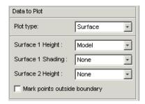
You can view any of these options alone as a primary surface (by leaving the last two options set to **None**). You can add a second option to shade the primary surface, for example to color your model surface with the error between the model and the strategy, to highlight problem areas.
