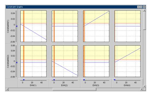
The Left Value is compared with a plot of the Right Value output on the same axes. This comparison is illustrated for the table gradient example problem. Consider the top-left graph in the figure shown. Constraint4(1) is the first Left Value  $(rg_1^{inc})$  of the table gradient constraint in the example problem. Recall that this can be written as
