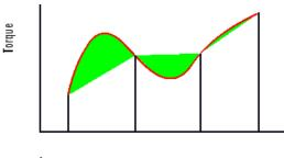
The green shaded areas show the error between the interpolated table values and the model using the initial breakpoints.
