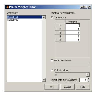
In this dialog box, you can select objectives to sum, and select weights for any run by clicking and editing, as shown in the previous example. The same weights are applied to each solution to calculate the weighted sums. Click  $\mathbf{OK}$  to apply new weights, and the weighted sums are recalculated.
