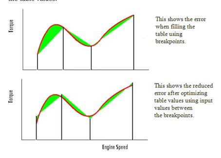
To see the difference between optimizing table values and optimizing the positions of breakpoints, compare with the illustration in "How CAGE Optimizes Normalizer Breakpoints" on page 4-5.
